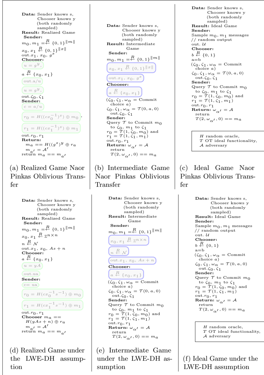
Diagram 9: Games 9a to 9c show the original Naor- Pinkas Sender security proof. A Chooser able to acquire both messages can solve the CDH problem. Games 9d to 9f depict the LWE-DH proof for the Sender. H denotes the random oracle.
